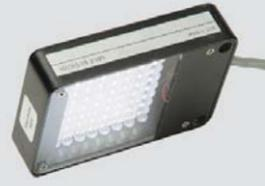
An Area Array's general purpose, unidirectional design (adjustable via mounting position) may be used for dark-field (creating shadows and specular reflection) or for bright-field lighting for diffused surfaces.
