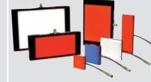
Backlights provide diffused illumination from behind the subject. Used to outline a part's overall shape, minimize visibility of clear housings, and to view openings such as drilled holes.
