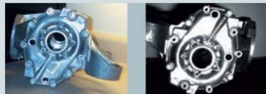
**Object: Housing assembly.** Detect presence/absence of fasteners.
