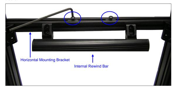
7. Using the 5/32" Allen key, insert the two (2) screws removed from the previous step into the screw openings on the docking plate.
