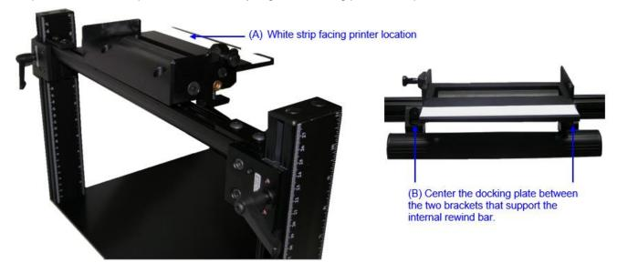
9. Using the 5/32" Allen key, tighten the screws to secure the docking plate to the horizontal mounting bracket.
