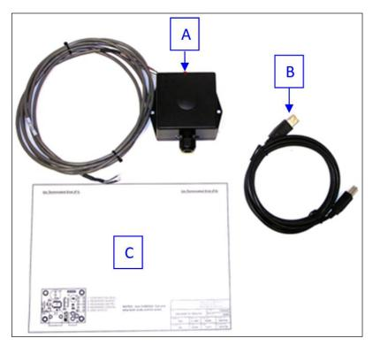
2. Mount the SMU to the desired location by inserting a screw (supplied by customer) into each flange located on the left and right side of the SMU. Hole size accepts an 8-32 or M4 screw.
