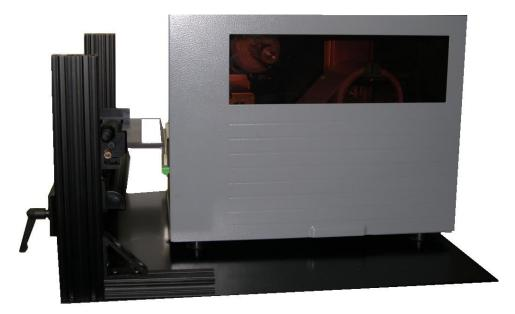
11. Adjust the height of the horizontal bar so that the docking plate aligns as close as possible to the height of the printhead. Do this by loosening the quick lock handle and then slowly adjust the horizontal mounting bracket so that the readhead fits snugly against the printhead. When the ideal position is located, tighten the quick lock handle. See correct and incorrect placement examples in the next section.
