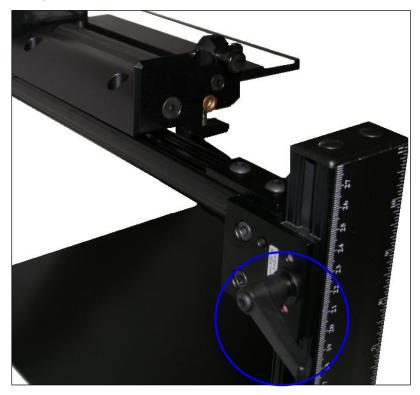
12. If the docking plate needs to move left or right to align with the printhead, simply loosen **(do not remove)** the two screws on the docking plate (using the 5/32" Allen key) and gently slide the docking plate to the ideal location. Then, tighten the two screws so that the docking plate secures firmly to the horizontal mounting bracket. See correct and incorrect placement examples in the next section.
