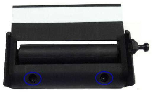
8. Place the docking plate on top of the horizontal mounting bracket with the white strip facing toward the printer location (see "A" below). Center the docking plate between the two brackets that support the internal rewind bar (see "B").
