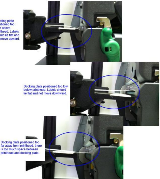
14. After the docking plate is correctly aligned with the printhead, gently pull out and turn the docking plate locking pin so that no part of the pin is visible.
