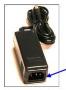
Plug one end of the AC line cord into the power supply box; plug the other end into a power outlet.
