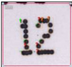
OCR Tool, dot matrix print, no image pre-processing, characters not well-segmented.
