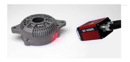
The 2D barcode reader smart cameras were installed at several stations through the facility. At each stage in the manufacturing process, 2D barcode reader reads the Data Matrix code and the data is sent to the host to verify that the component passed the previous steps before proceeding to the next station.
