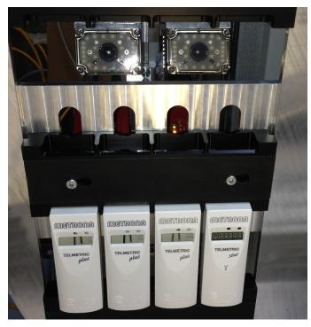
Microscan's Vision HAWK smart cameras ensure that the Data Matrix codes are correct and readable on the heat cost allocators from BRUNATA-METRONA.
