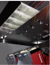
The Vision HAWKs read the codes using a job created with AutoVISION® machine vision software and send the data back to BRUNATA-METRONA's central system for control. No PC or additional lighting is needed.
