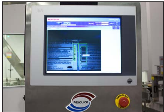
Microscan's Visionscape I-PAK software displays inspection results on an HMI screen.
