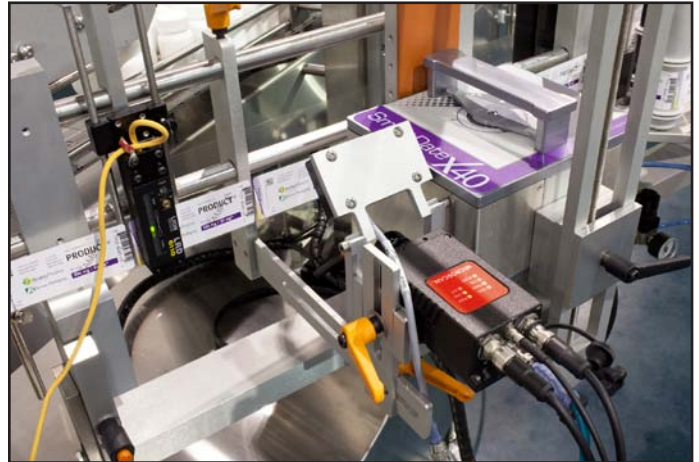
Microscan's VS-1 smart camera verifies labels before they are applied to containers.
