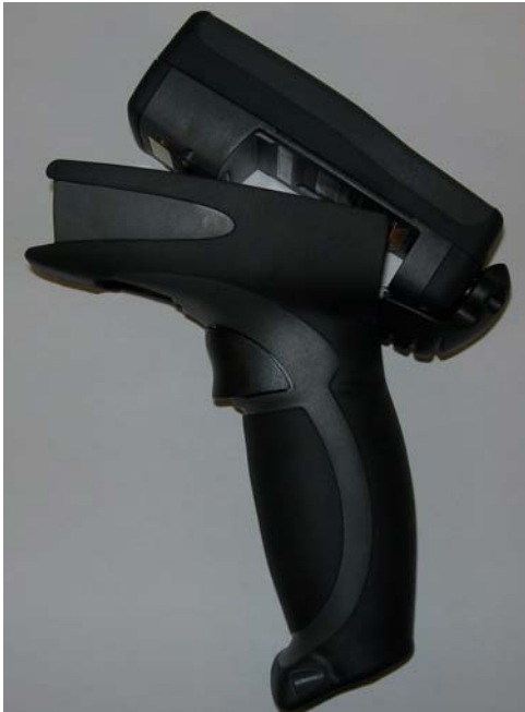
FIGURE 1–4. Attaching the H2 Handle
