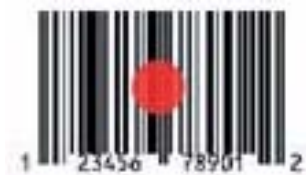
FIGURE 1–38. Centering the Symbol Within the Laser Dot
