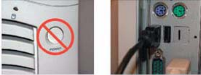
FIGURE 1–15. Installing the USB Cable
