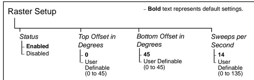
Figure 2-7 Raster Setup Menu Structure
