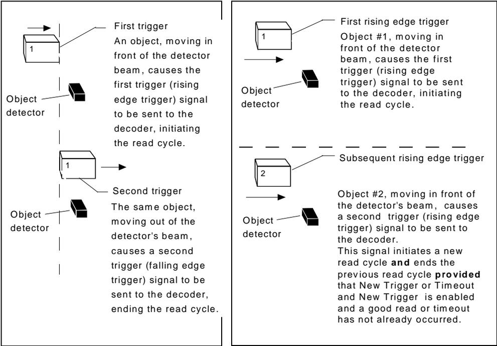
Figure 2-1 External Level Trigger Signals
