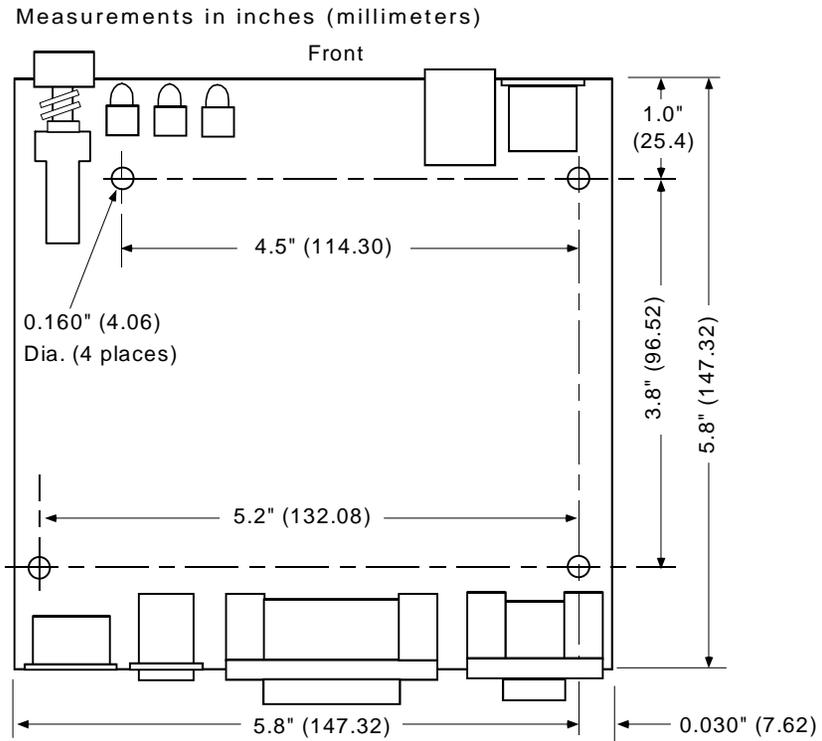
Figure 1-13 Mounting Diagram (without housing, not full size)
