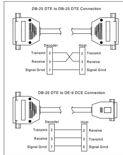
Figure 1-10 DTE and DCE Host Connections
