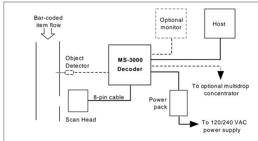
Figure 1-1 System Diagram
