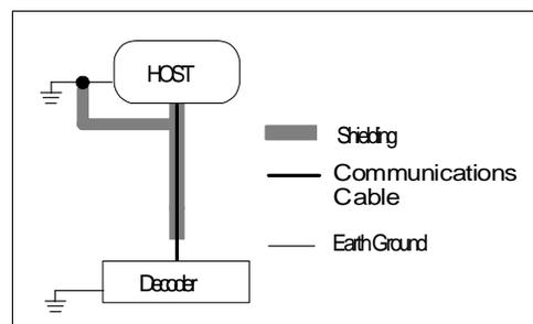
Figure 1-14 Grounding Diagram, Decoder-Host
