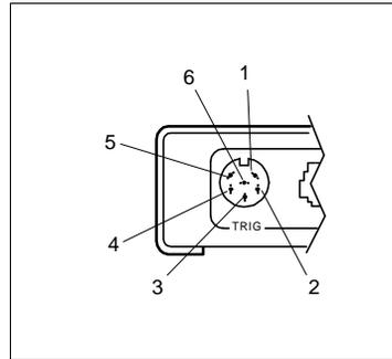
Figure 1-3 Trigger Connector Socket
