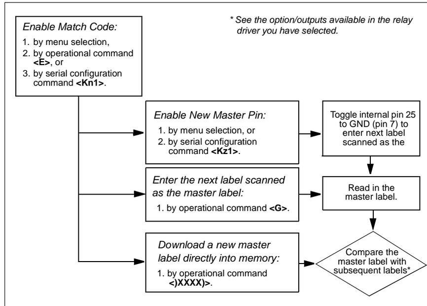
Figure 2-4 Match Code Logic Diagram
