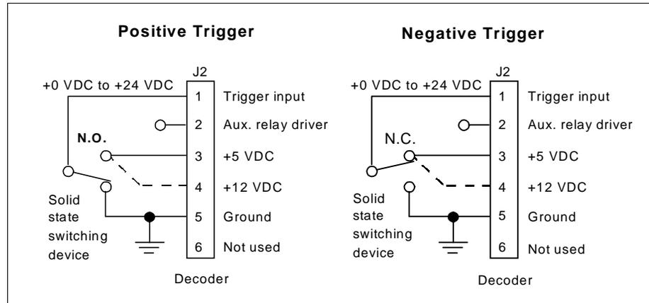
Figure 1-4 Trigger Connector Wiring Diagram (untriggered)
