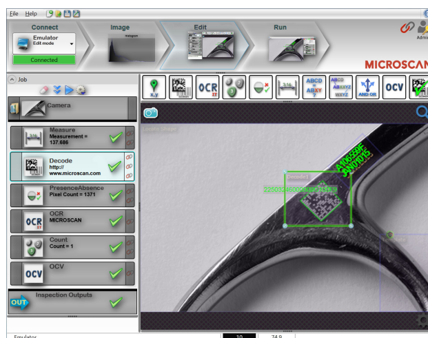
Microscan's AutoVISION® Machine Vision Software decodes direct part marks using X-Mode algorithms on the connected camera.
