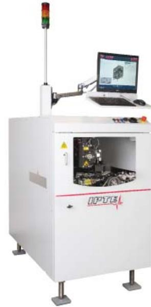
**The ultra-compact MINI Hawk barcode readers are integrated inside the in-line laser marking solutions from IPTE.**
