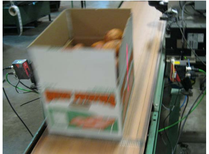
Pack codes are scanned with QX-830s to confirm product type. This data is used to generate PTI-compliant labels.
