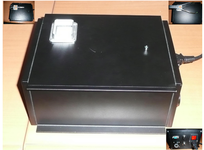
The CIP 2D-DPM reader from CIPAM allows users to read laser and dot peen 2D DPM markings from all metal surfaces.
