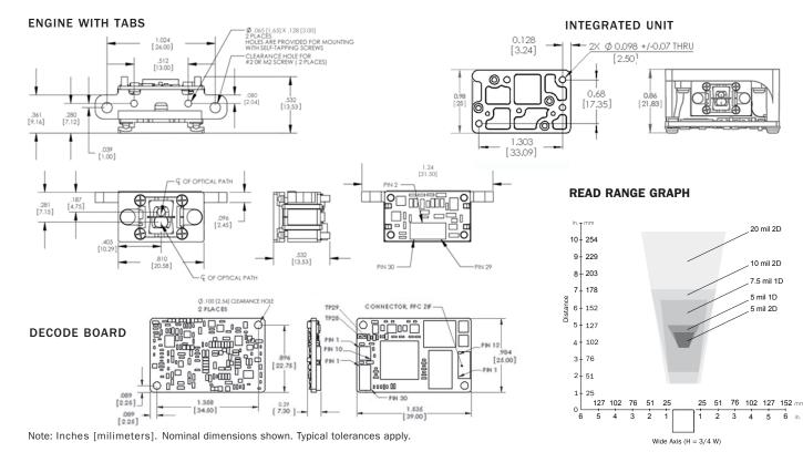
**MECHANICAL (ENGINE) Height:** 0.47" (11.9 mm) **Width:** 0.81" (20.6 mm) **Length:** 0.57" (14.5 mm)
